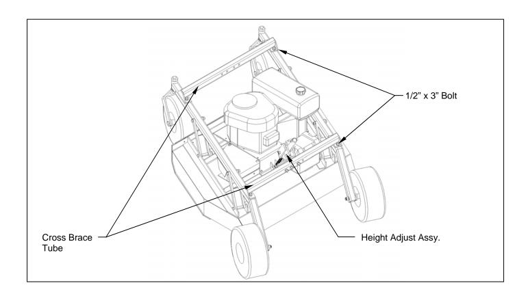
Figure 3: Cross Brace Tube Installation
